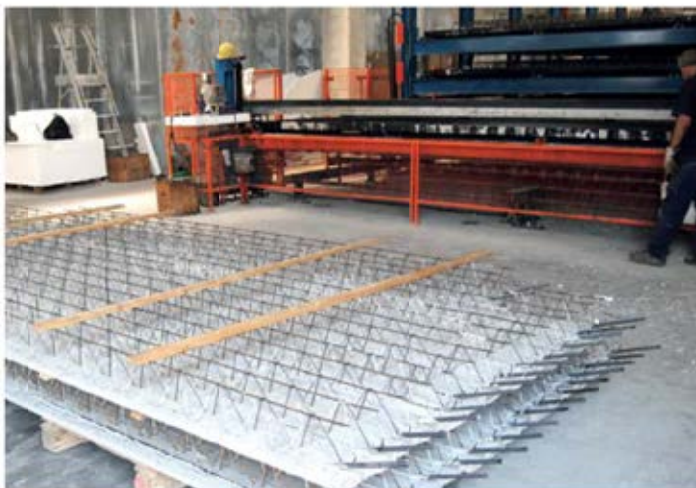
← Beams in two side-by-side rows, to form a double-width stack.
