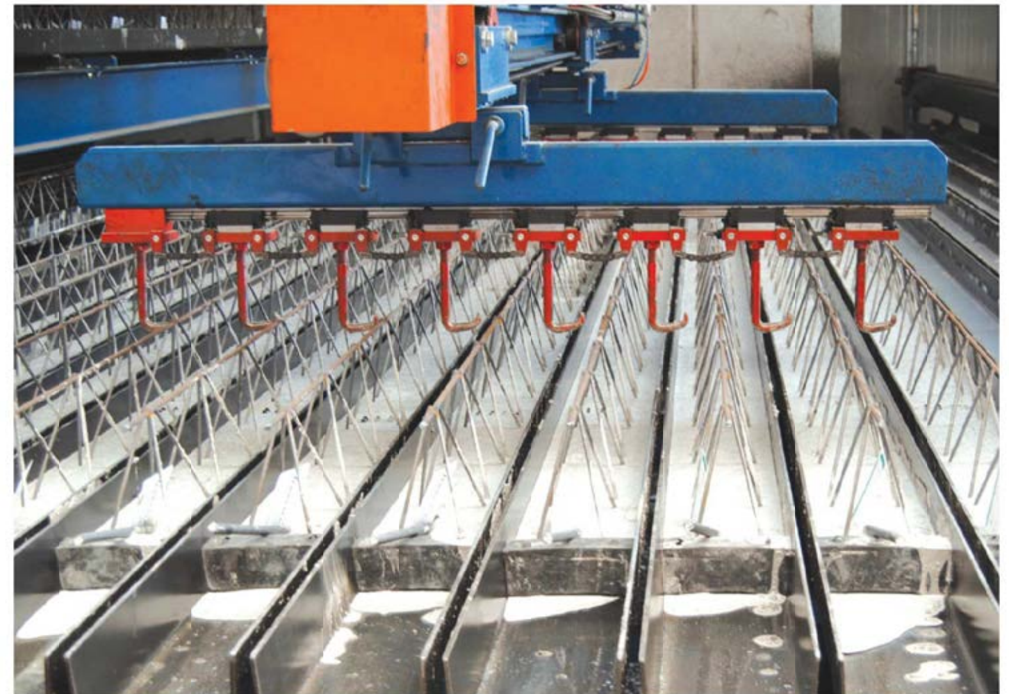
↓ Stacking clamps in the clamping stage for picking.
