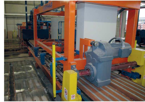
← Elephant, self-propelled carriage with shakeout clamps.
