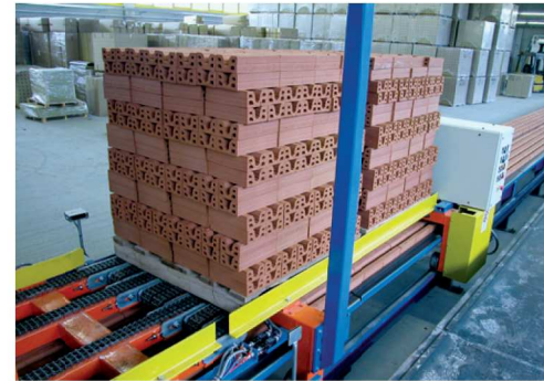
← Jolly carriage, self-propelled, operates automatically.
