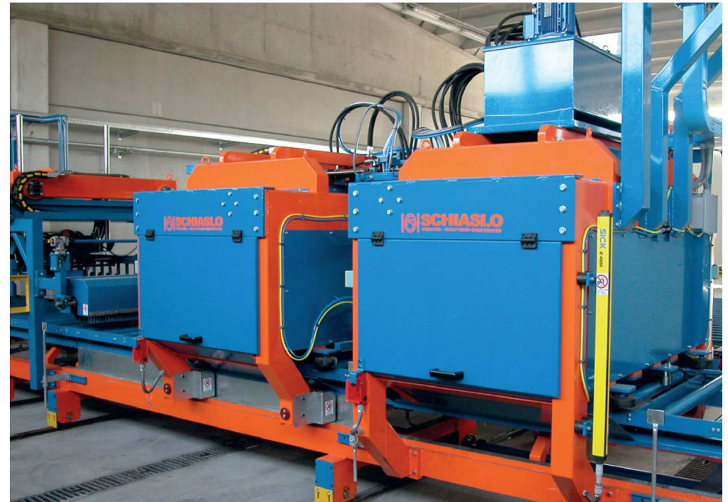
↓ Automatic cutting device, with one fixed and one mobile station.
