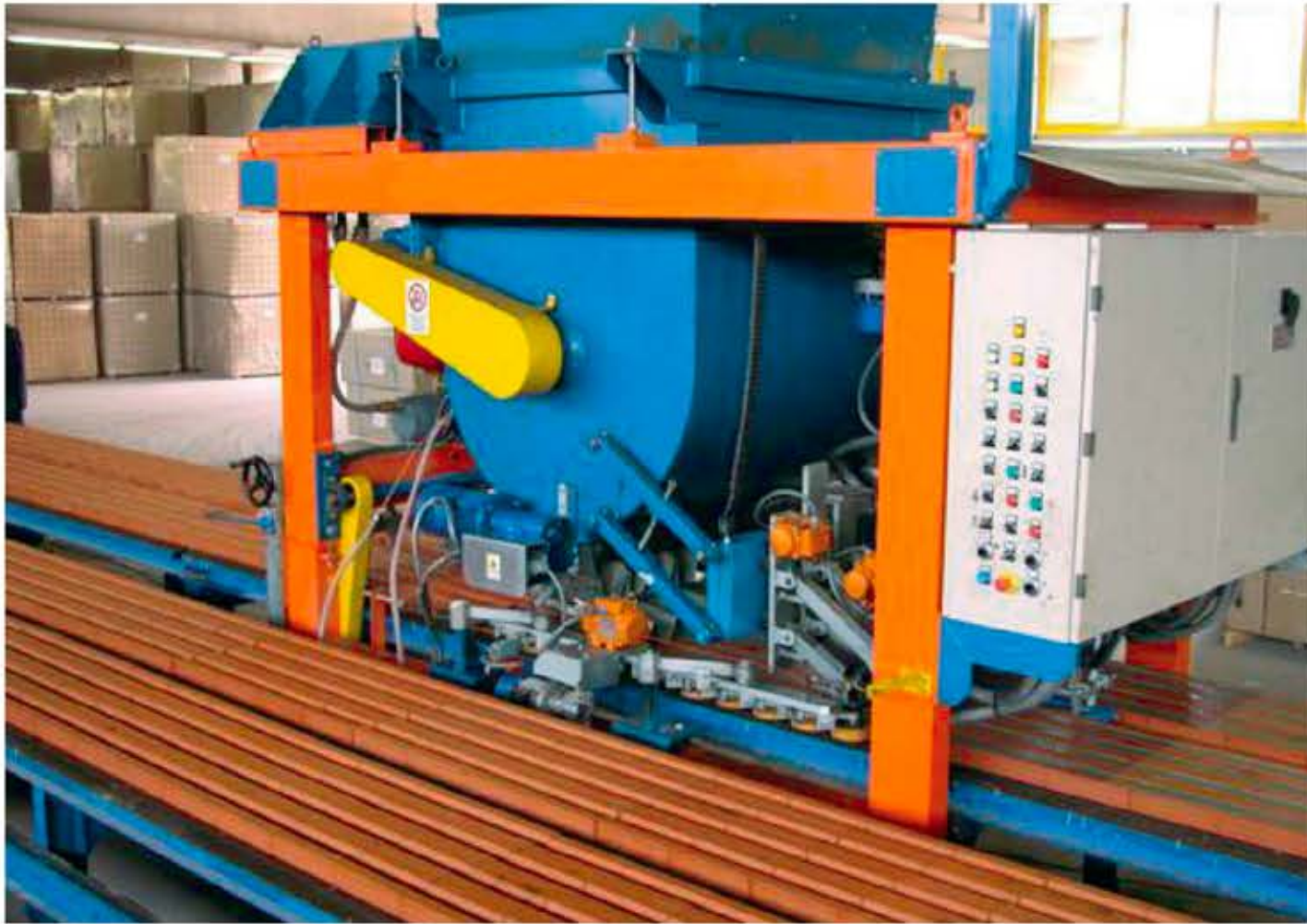
↑ Batching carriage in casting stage, operates with one worker only.
