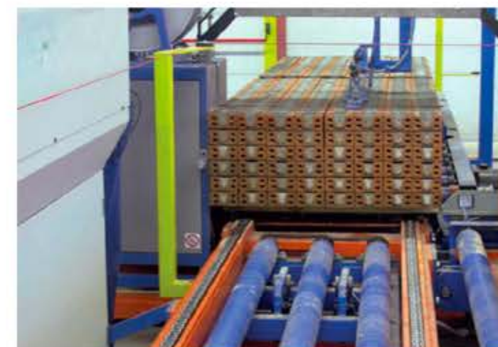
← Operation of automatic strapping of a stack of lintels, 12cm wide.
