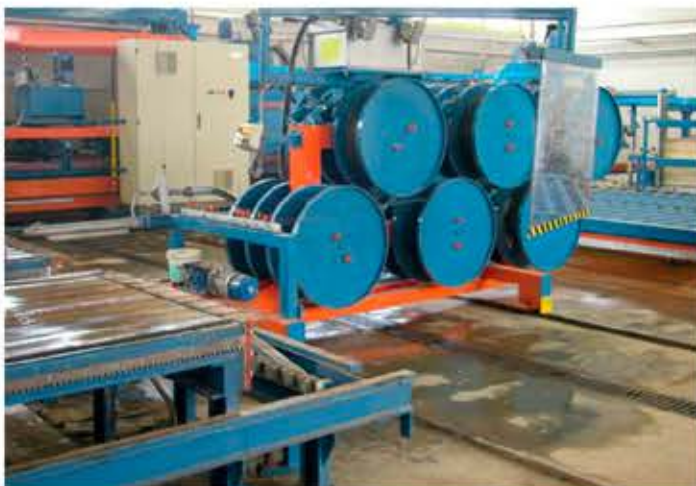
← The reel carriage, motorised.
