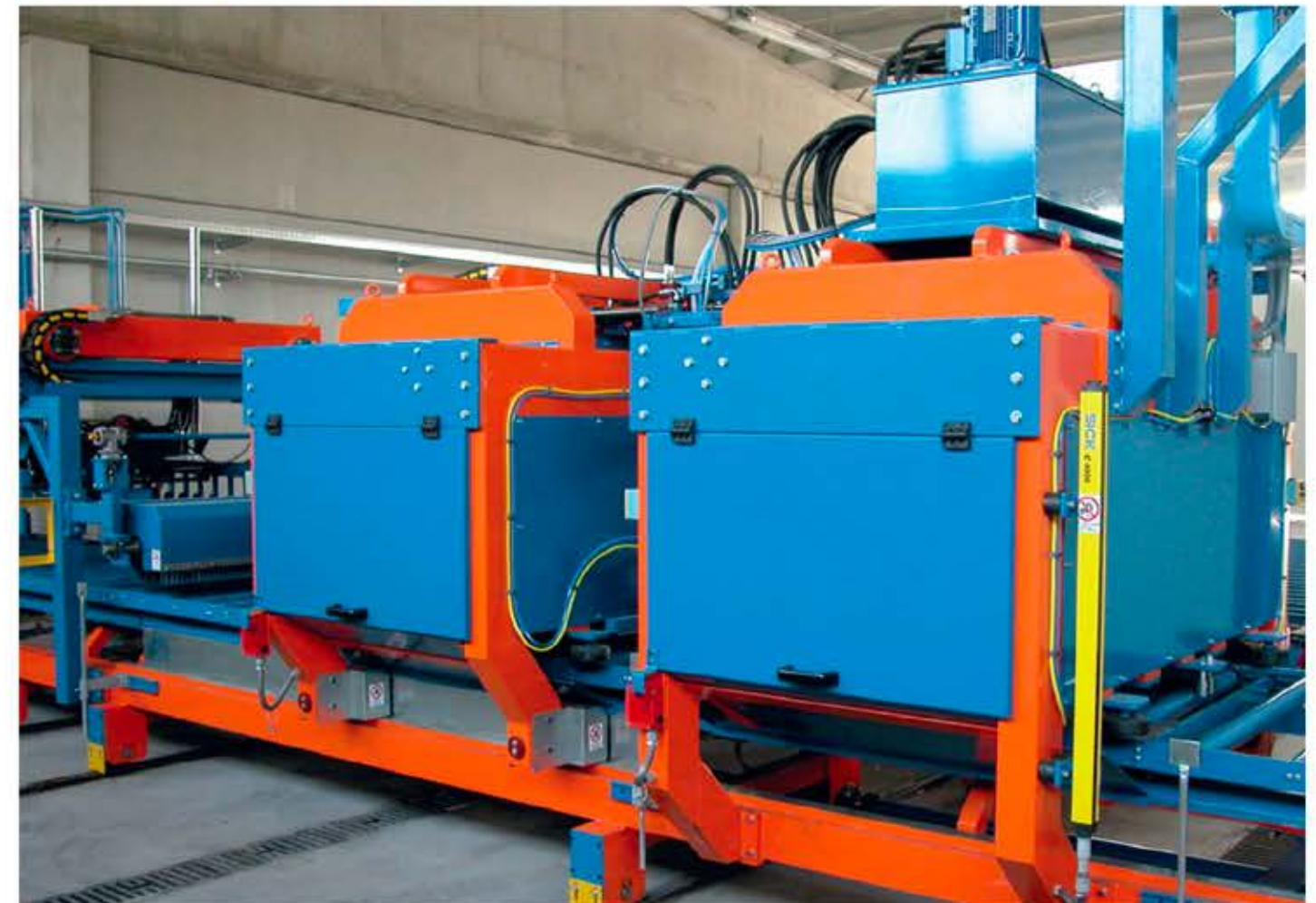
↓ Automatic cutting device, with one fixed and one mobile station.
