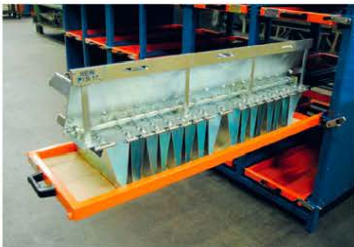
← Interchangeable distribution hopper.
