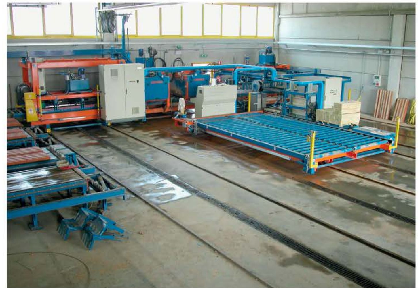
↑ Multifunction self-propelled carriage.
