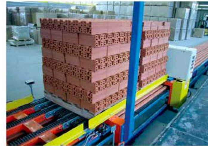
← Jolly carriage, self-propelled, operates automatically.
