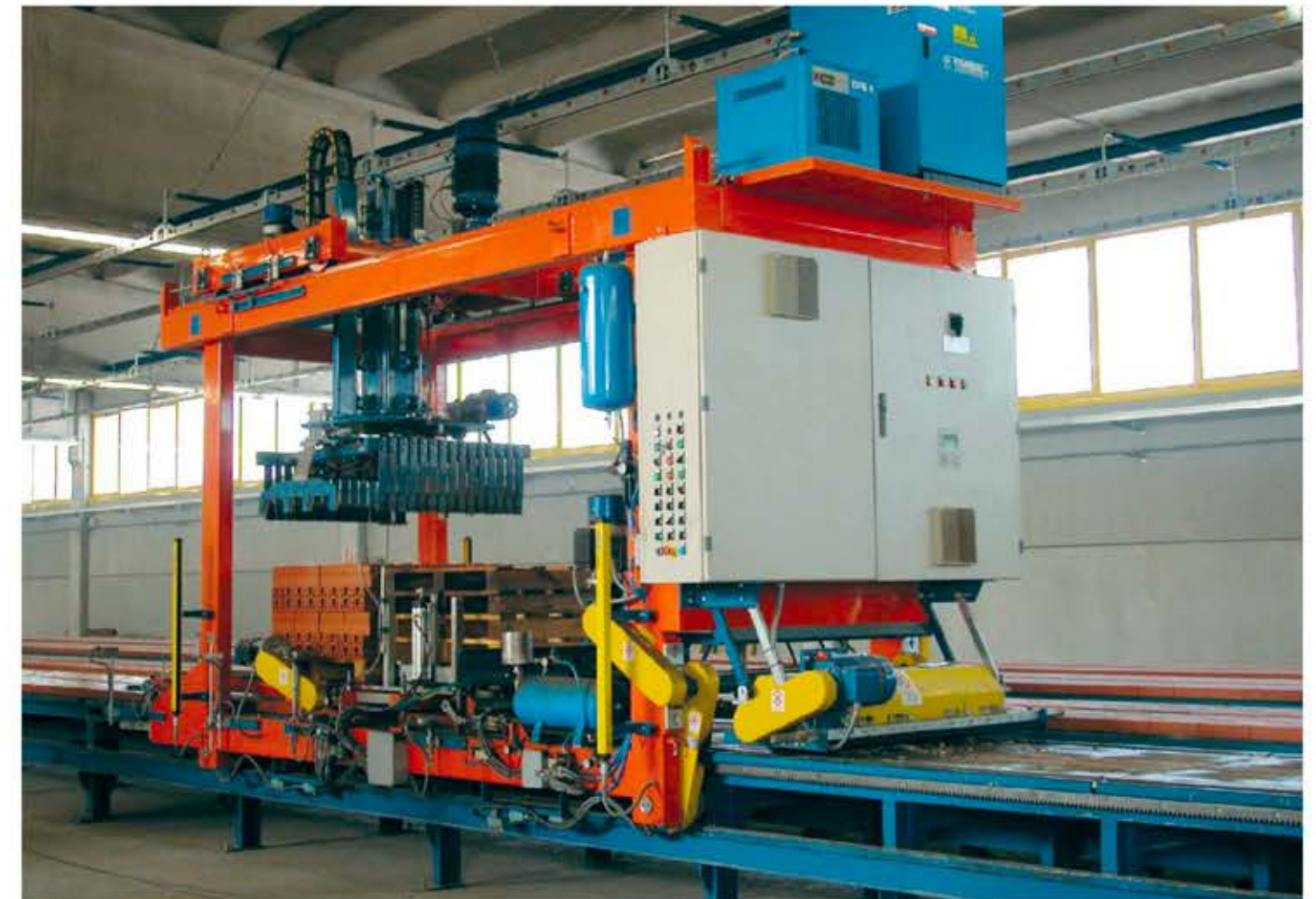
↓ Brick laying carriage, operates with one worker only.
