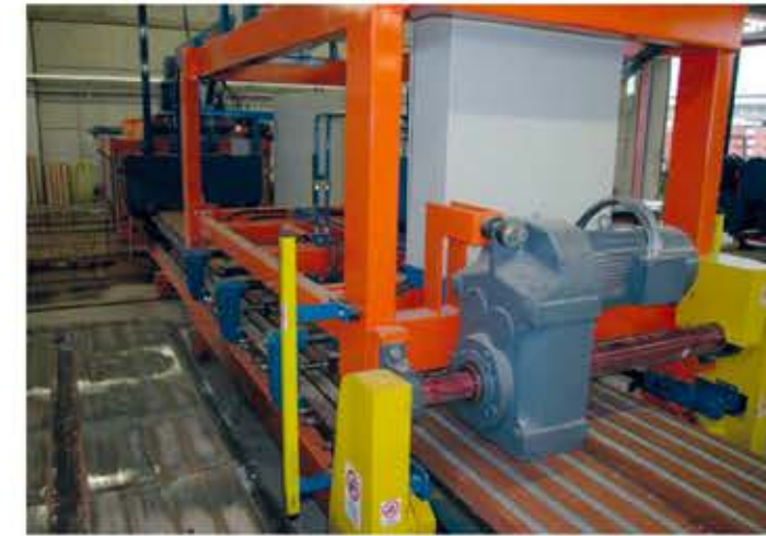
← Elephant, self-propelled carriage with shakeout clamps.
