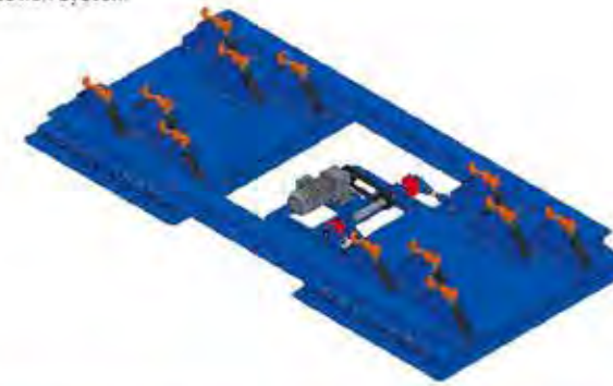
REF. 07/ Noiseless platform vibro-compaction system
