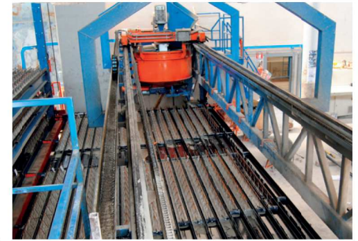
→ The self-propelled batching carriage, on its own overhead track.
